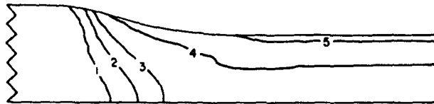
b. 30% reduction (Interval between contours = 12 MPa ; Contour 1 = 66 MPa)
