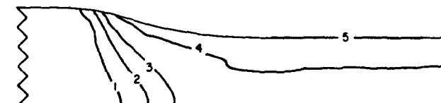
b. \theta_0 = 560 K (Interval between contours = 12 MPa ; Contour 1 = 66 MPa)
